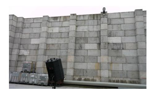
Based on sound reduction measurements in field situations (report 171402a of 20 December 2023), the following sound insulation values have been determined for the Legioblock wall system.
